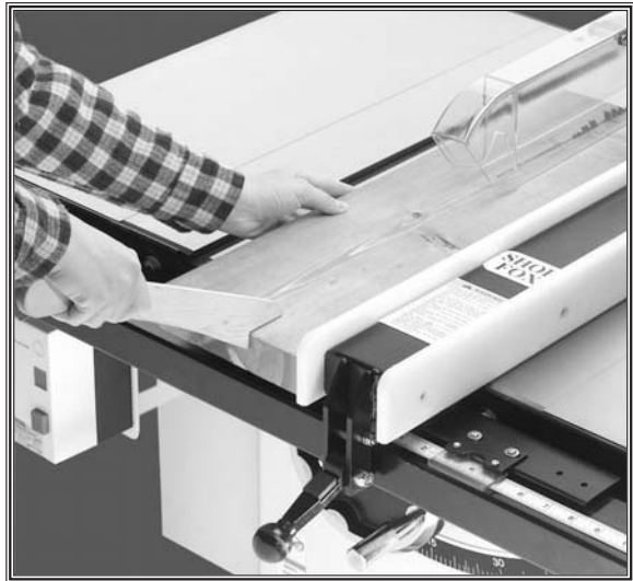
Figure 51. Typical ripping operation.
